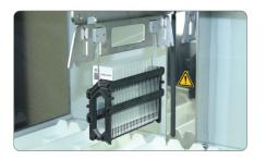
Loading up to 30 slides simultaneously
